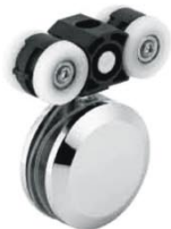
GLX-7034 Sliding door wheel Maximum loading: 120 kg Door thickness: 10-12mm
