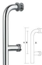
GLX-3056 Material: Stainless steel Finish: PSS/SSS Size(mm) A:300 B:200 D:Φ25
