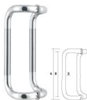
GLX-3052 Material: Stainless steel Finish: PSS+SSS Size(mm) A:625 B:600 D:Φ32
