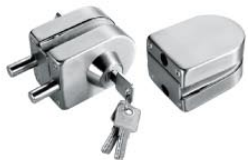
GLX-9026 Materials: Stainless steel / Iron Finish: Chrome,Satin Door thickness:10-12mm Tempered glass door
