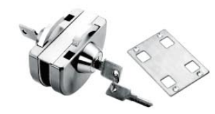
GLX-9008 Materials: Stainless steel / Iron Finish: Chrome,Satin Door thickness:10-12mm Tempered glass door
