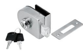
GLX-9033 Materials: Stainless steel / Iron Finish: Chrome,Satin Door thickness:10-12mm Tempered glass door
