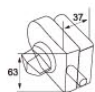
GLX-9039 Materials: Stainless steel / Iron Finish: Chrome, Satin Door thickness: 10-12mm Tempered glass door
